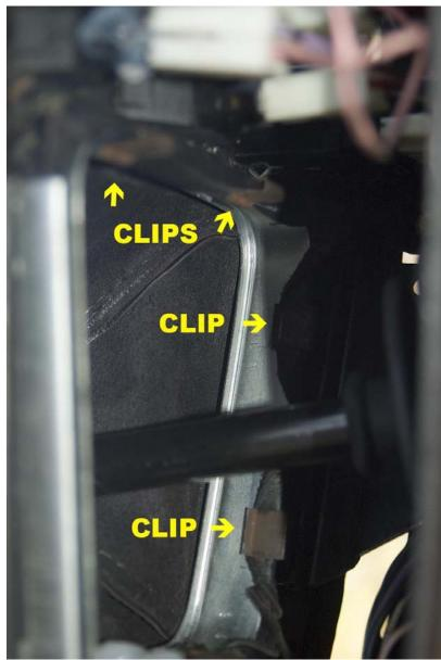
The leather boot is secured with a bunch of clips
