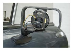
Step B) SEE PICTURES Once the cover is off you can gently pry-off the mirror. The actual mirror is attached with 4 plastic snaps.
