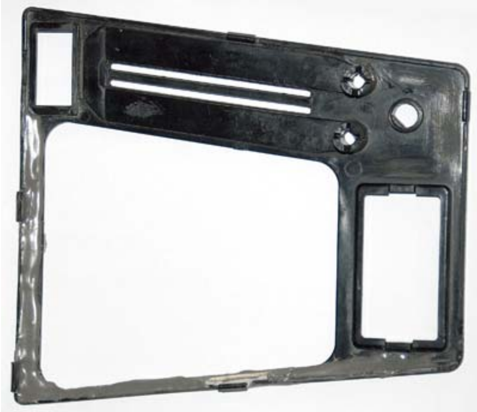
Nails are embedded with JB Weld
